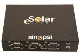
eSolar LIGHT is a system for monitoring and managing local or remote maintenance of photovoltaic plants of size not exceeding the 50kWp and / or up to 10 inverters (inverters must be all of the same brand).
